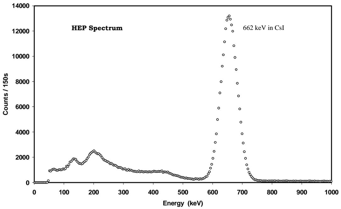
Figure-3 : Simultaneous recording of LEP & HEP spectrum with <sup>137</sup>Cs source
