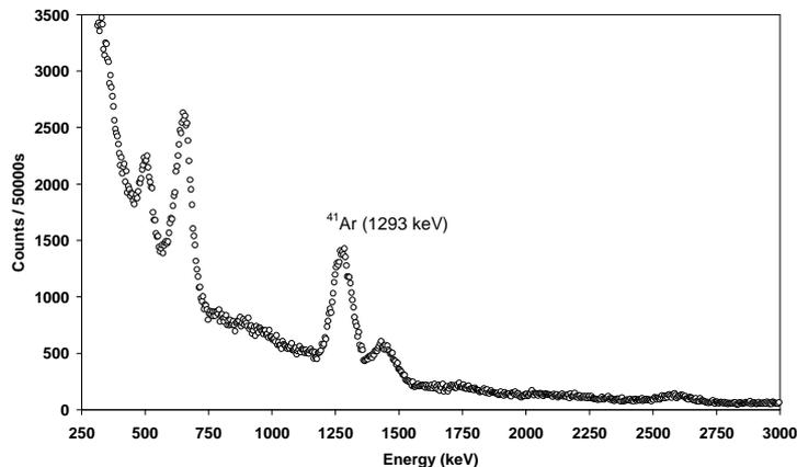
Figure-5 : HEP spectrum during  $^{41}\text{Ar}$  interference
