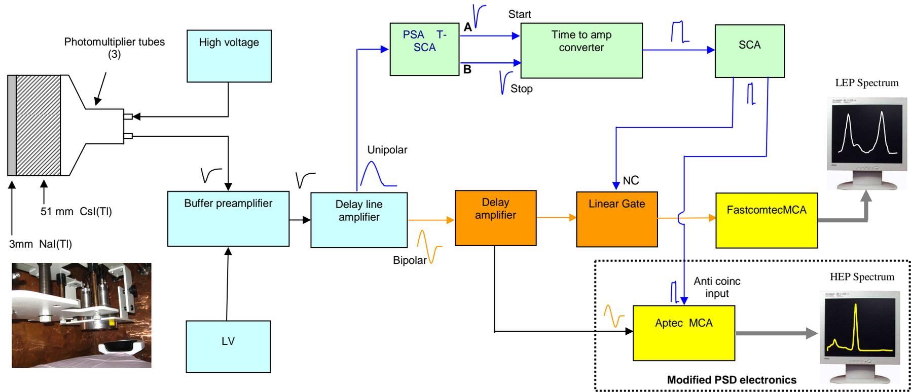
Figure-1: Phoswich PSD electronics for simultaneous recording of HEP & LEP spectrum
