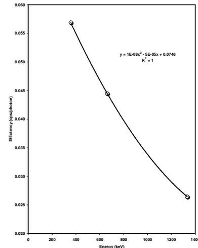
Figure-2: Point source efficiency
