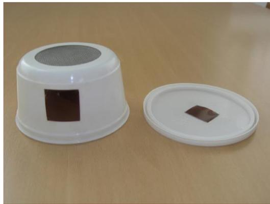
**Figure 1.** Plastic vessel with placed diffusion (on the right) and open (to the left) LR 115 type II detectors.
