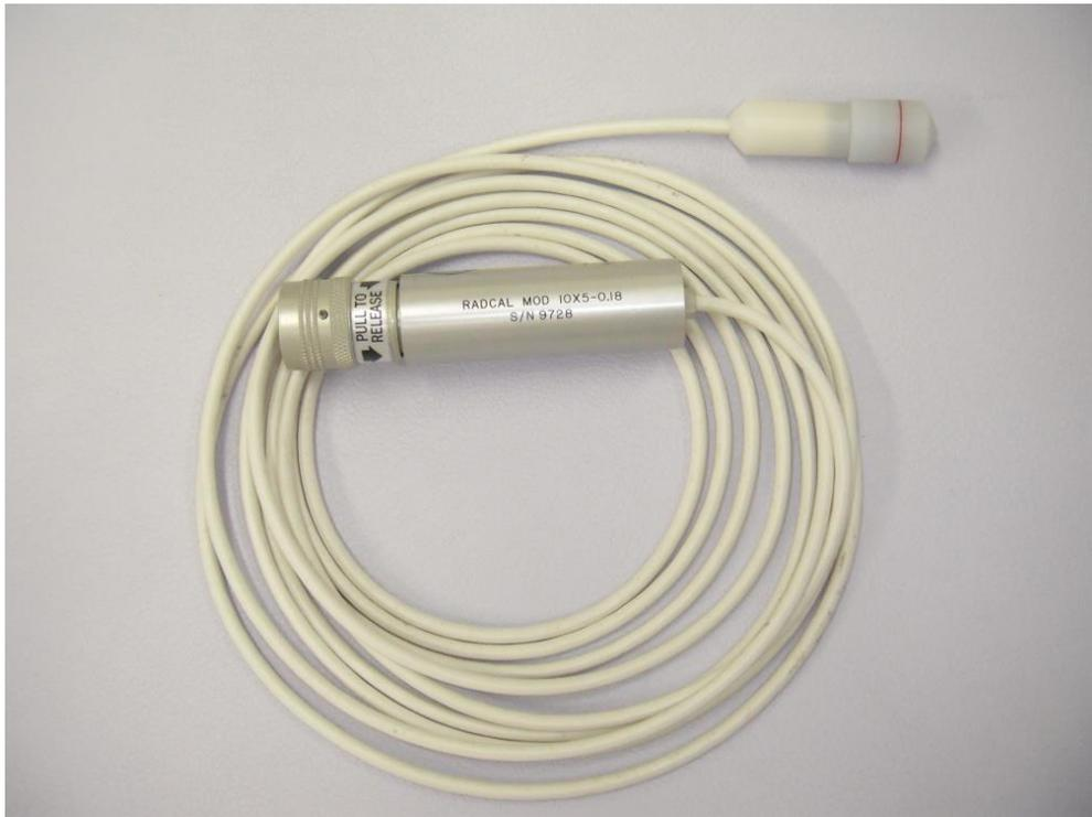
**Fig. 1 10X5-0.18 Micro Ionization Chamber**
