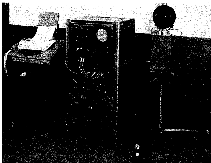
FIG. 7. Component of LET system as used in field measurements. Rack cabinet contains, from top to bottom, the 400 channel pulse height analyzer, the ETC chassis containing amplifier, clipper, router and preamplifier power supply, the analog computer, a high voltage power supply, and a test pulse generator.
