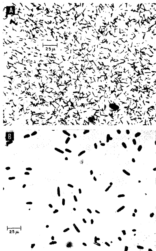
FIG. 5. Fission fragment tracks in Lexan. (A) High track density ( \sim 4 \times 10^6 \text{ cm}^{-2} ) and short etching time (5 min). (B) Lower track density ( \sim 10^5 \text{ cm}^{-2} ) and longer etching time (40 min).
