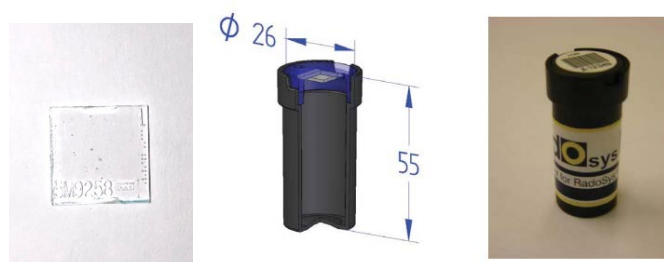
Figure 3. Radosys CR39 detector chips (with and without chamber) (RADOSYS© User Manual)
