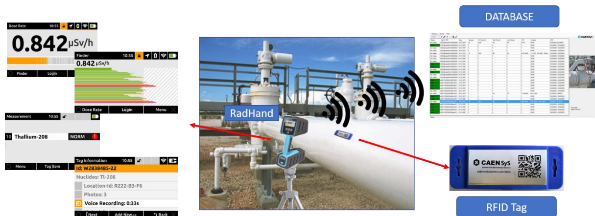
Figure 6: Example of normal operation during pipe section or valve inspection procedure with Digiwaste in NORM management process for Oil & Gas Industry.
