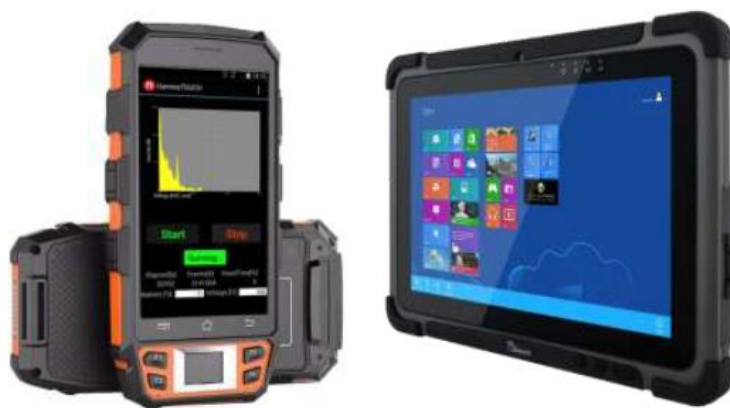
Figure 5: Ruggedized, Portable UHF RFID Readers. These devices provide operators not involved in nuclear measurements with access to the central database and UHF RFID tags.
