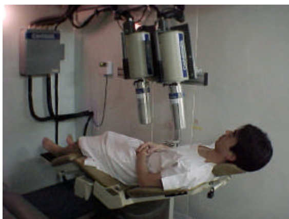
Figure 1 JNC-Whole body counting system with Ge detectors, installed in the special shielding room
