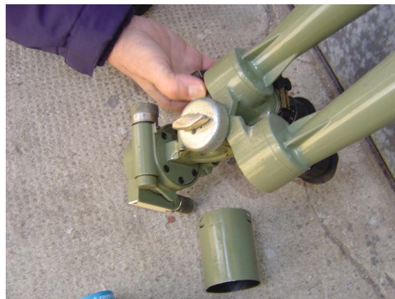
Figure 5. A typical military item with non-registered Ra-226 source inside it. No label related to radioactivity was used at the time the equipment was acquired.
