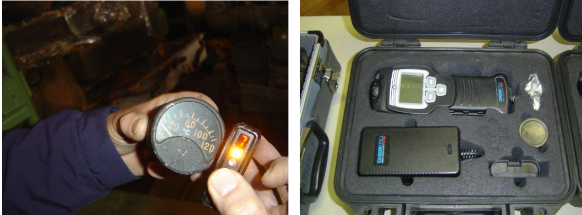
Figure 4. Two types of non-registered sources, namely Ra-226 radioactive paint used in an old instrument causing a dose rate more than 9 \mu\text{Sv/h} (left) and a new instrument with 6 MBq Am-241 installed in a ChemPro gas analyser (right).
