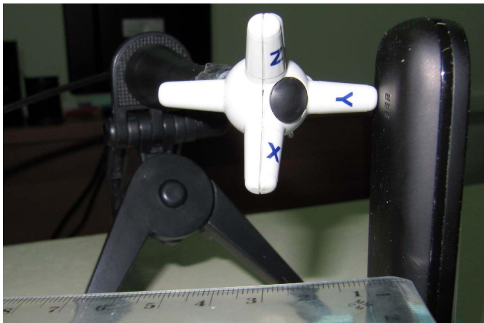
Figure1 Experimental setup. Here the 3-axis electric field probe 'sees' the rear side of phone.
