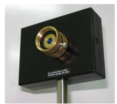
Figure 3, the artificial eye method measurement device
