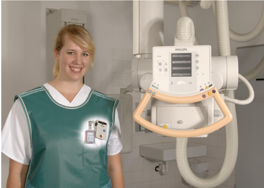
Figure 1: Active electronic dosimeter in a typical pulsed radiation field used at medical diagnostic X-ray units. The protective clothing has been made invisible at the position of the dosimeters to show the correct position of the dosimeters (film dosimeter as the legal dosimeter and an additional electronic direct reading dosimeter).
