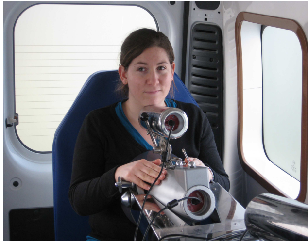
Figure 3: whole body and thyroid measurement of a subject in the emergency minivan
