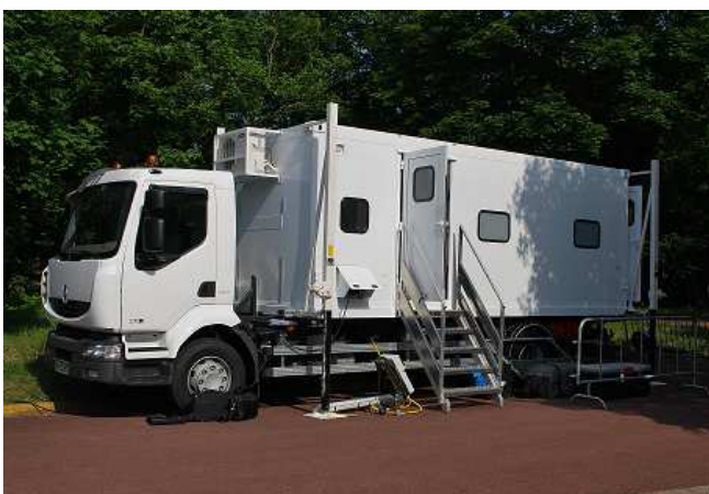
Figure 4: General view of the heavy emergency mobile unit (the shelter is placed on its truck for road transportation)
