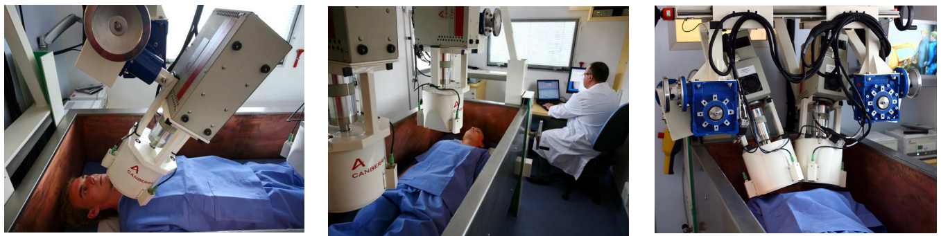
Figure 8: Inner view of the expertise mobile unit. Left: thyroid measurement, middle: whole body measurement, right: lung measurement
