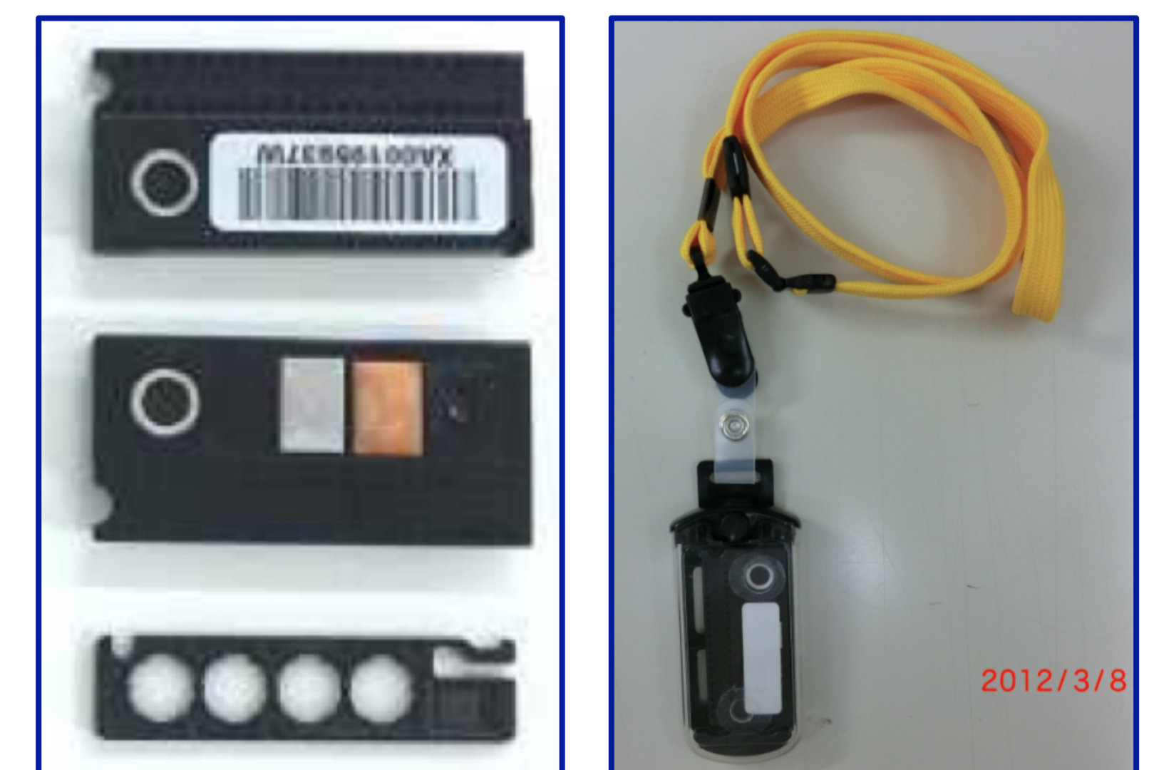
Fig.2 InLight badge system (left) and a badge worn on a neck strap (right).
