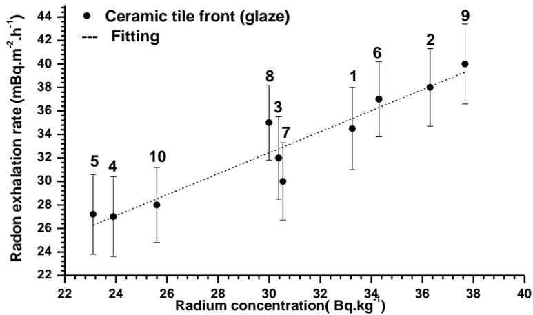
Fig.4.The dependence of the radon exhalation rate from the glazed side on the <sup>226</sup>Ra concentrations of floor tiles.Numbers with each point indicate the source manufacturers.
