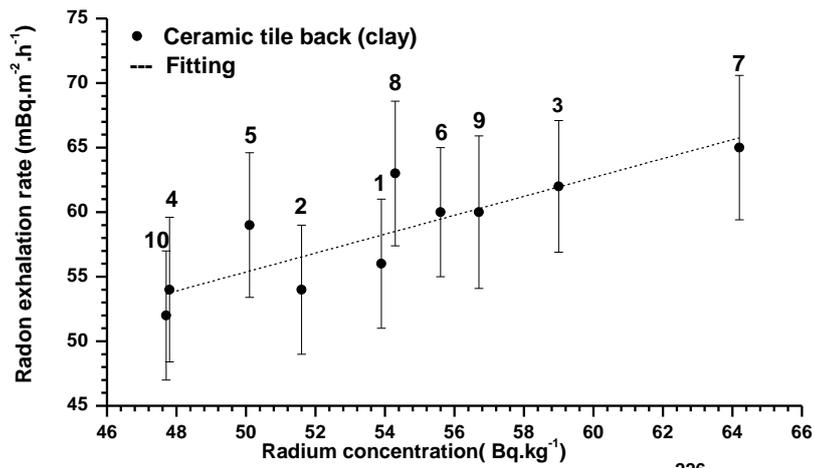
Fig.5.The dependence of the radon exhalation rate from the clay side on the <sup>226</sup>Ra concentrations of floor tiles. Numbers with each point indicate the source manufacturers.
