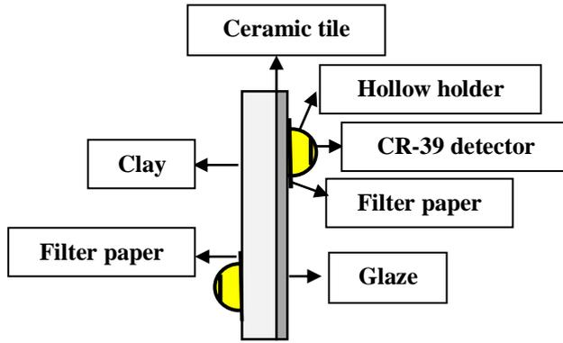
Fig. 1. The setup diagram for measuring radon exhalation rate of ceramic tile.
