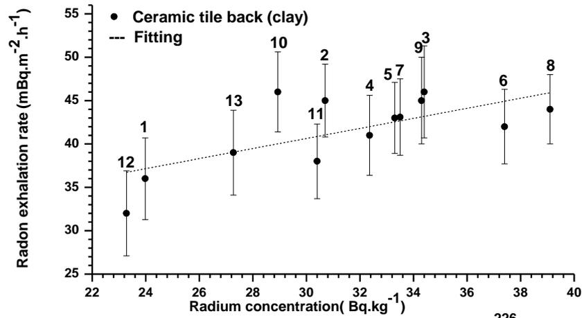
Fig.3.The dependence of the radon exhalation rate from the clay side on the <sup>226</sup>Ra concentrations of wall tiles.Numbers with each point indicate the source manufacturers.
