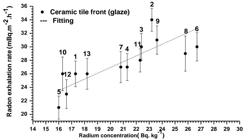
Fig.2. The dependence of the radon exhalation rate from the glazed side on the <sup>226</sup>Ra concentrations of wall tiles. Numbers with each point indicate the source manufacturers.
