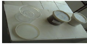
Preparation of stone samples with Marinelli Beakers
