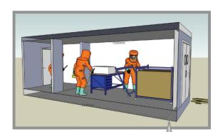
The operation is undertaken in a rigid, ventilated containment facility.
