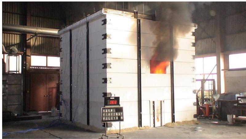
Figure 3. Compartment fire test
