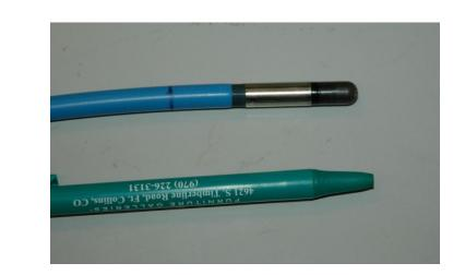
A 0.125 cc PTW pencil ion chamber (right bottom) and Keithley 35050A dosimeter (right top) were used to measure the air kerma in pico-coulombs. Once the phantom was created, dose data were collected in the brain of the canine phantom for two configurations: (1) with the head in the primary beam, (2) with the chest in the primary beam. The doses were measured at commonly practiced CT
