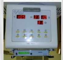
Figure 4: DAP meter mounted onto light beam diaphragm of x-ray tube
