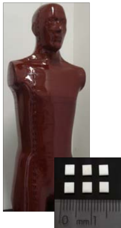
Antropomorphic Alderson phantom, thermoluminescent dosimeters (left), standard body CT PMMA phantom and pencil CT ionization chamber (right) used for CT dose measurements.
