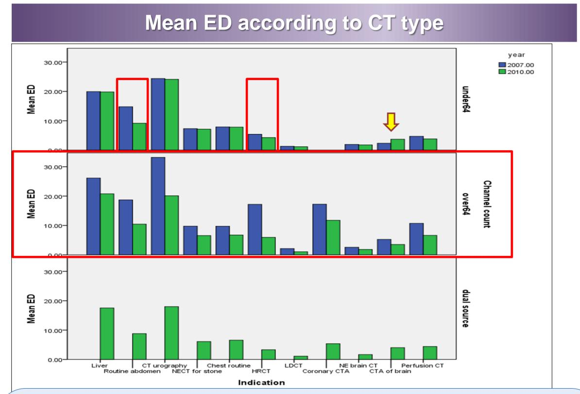
We divided CT machines into three types, CT with fewer than 64 detector rows, CT with 64 or over detector row and dual source CTs. At 2007, CT with 64 or more detector rows showed higher ED than CT with fewer than 64 detector rows. But at 2010, the EDs of each protocol become similar in variable CT machines. Generally dual source CT shows lowest ED in all protocols. In all protocols, CT with 64 or more detector rows showed significantly decreased radiation dose (red boxes).
