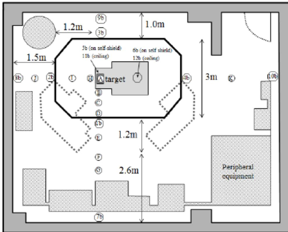
Figure2. Arrangement of glass dosimeter and gold foils in the PETtrace cyclotron room.
