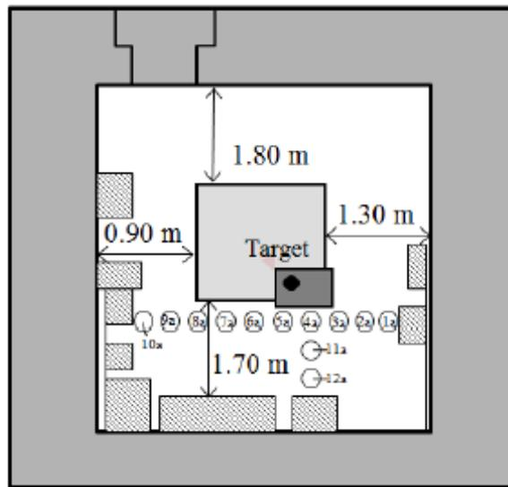
Figure 1. Arrangement of glass dosimeter and gold foils in the HM-18 cyclotron room.
