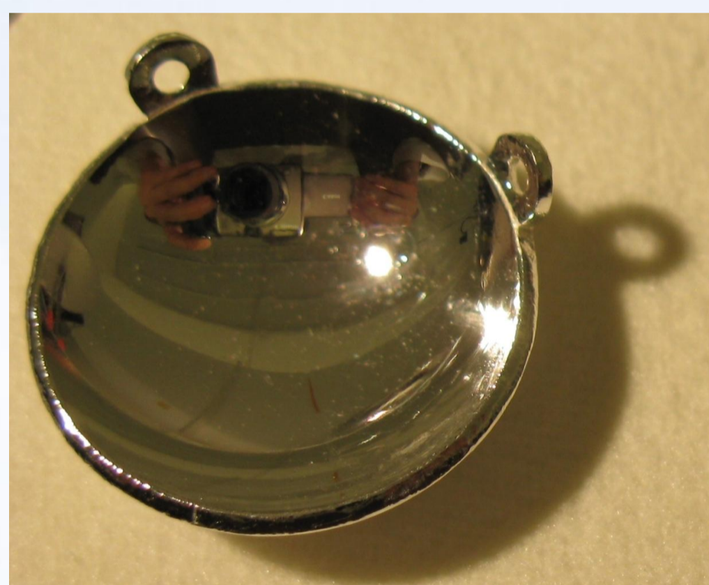
Figure 2: Typical Bebig Ru106 Eye Plaque Brachytherapy Source
