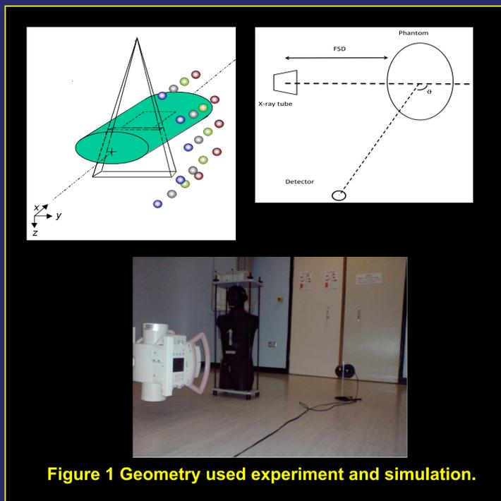
Figure 1 Geometry used experiment and simulation.
