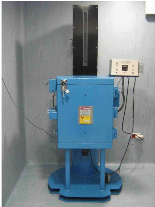
Fig.1a. A biological gamma irradiator
