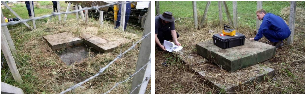
Figure 2: Buried source site with and without the concrete block shielding in place.
