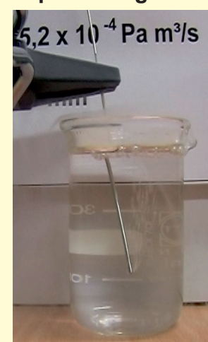
Bubble stream induced by a leak specified by a Standard He-Leakage rate of 5.2 \times 10^{-4} \text{ Pa}\cdot\text{m}^3/\text{s}
