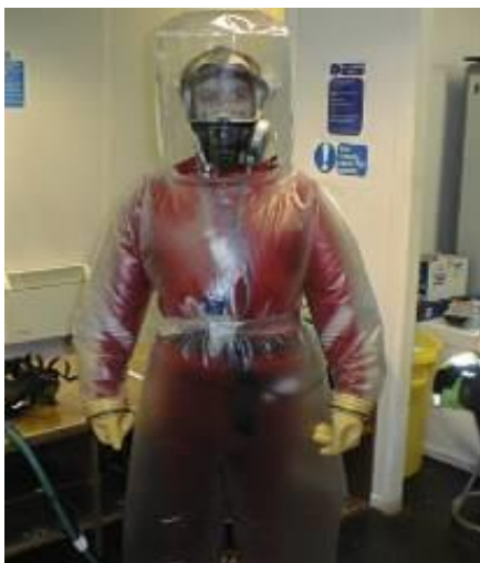
Figures 16(a) and 16(b) The Dounreay single use one piece Air Fed Suit with on built respirator
