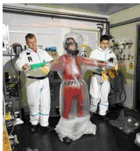
Figures 16(a) and 16(b) The Dounreay single use one piece Air Fed Suit with on built respirator
