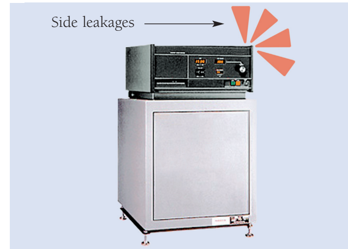
X-ray generator in self-shielded enclosure
