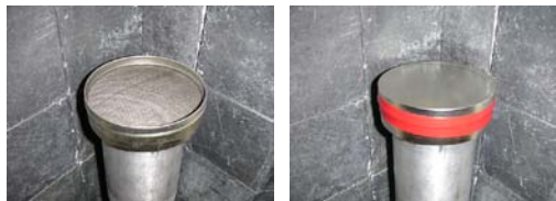
Figure 1 Photographs showing (left) open charcoal canister on top of the NaI detector (right) closed charcoal canister on the detector.
