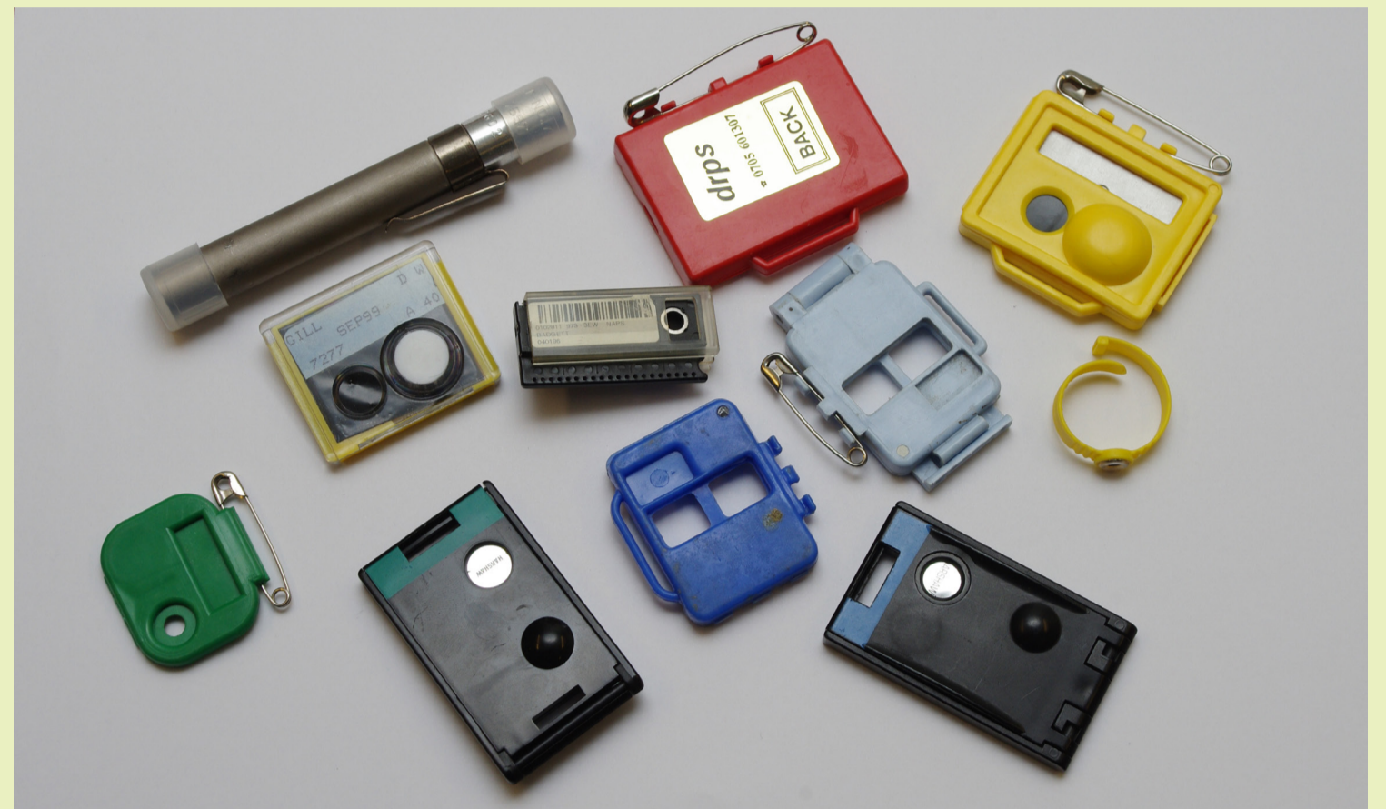
Fig 3: Examples of dose meters past and present
