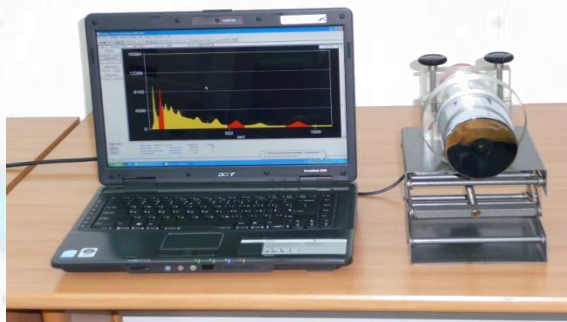
Fig. 1. The portable unit with scintillation detector NaI(Tl) for measurement of I-131 and Tc-99m
