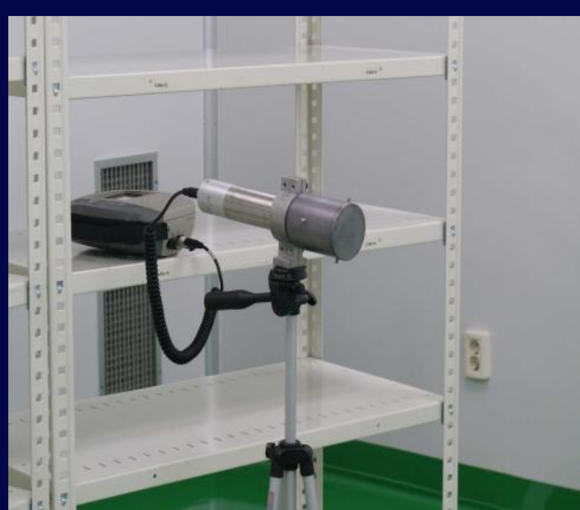
The portable NaI scintillation counter (left) irradiated by Cs-137 source for calibration and its MCNPX modeling (right)
