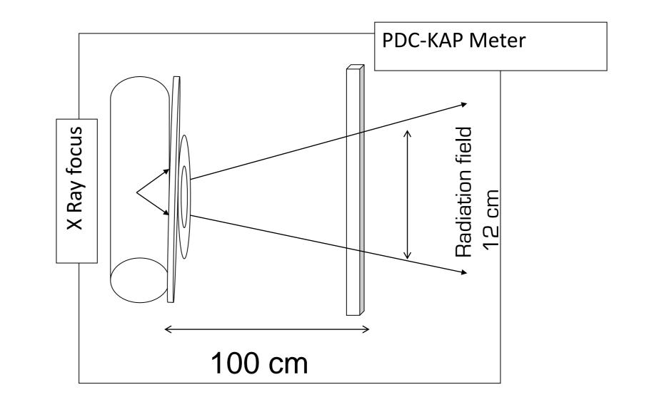
Set up used to measure the parameters Schematic view of the geometry used
