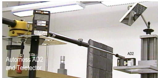
Fig. 2: The Automess 6150 AD2 and Teletector use Geiger counters. k_n was measured by means of a lead shield blocking photons from the neutron sources.
