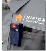
In addition to improvements in measurement capabilities, the DMC 3000 also has enhanced alarm capabilities, alerting users through the use of **vibrating alarms, dual LEDs and a high-decibel speaker**.
