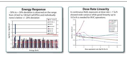
The first major improvement is the DMC 3000's energy and angular response, which remains flat from **16 keV to 7 MeV** without any deviances for angles up to +/- 60°.
