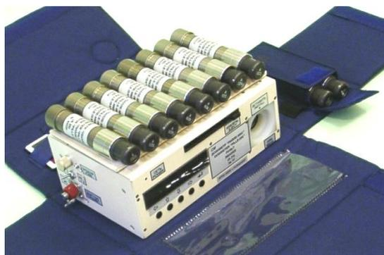
**Figure 1** The Pille TL dosimeter system in its transporting case (reader and ten dosimeters)
