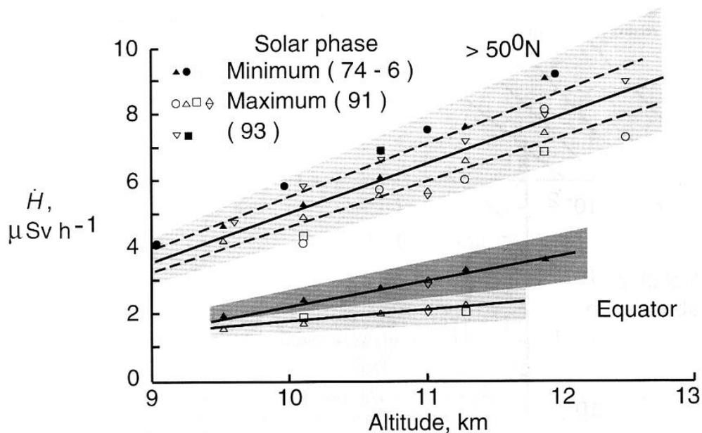
**Figure 3** The typical values of total dose equivalent rates in the supersonic flight altitude range
