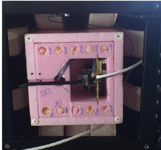
**Figure 7 The measurement geometry in the CoCoRAD experiment (in the holes with numbers indicated where the Pille bulbs can be found inside the thermal insulation and a mechanical protection aluminium box)**
