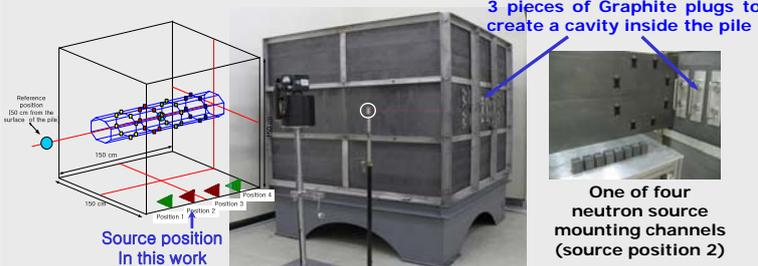
Graphite pile and Neutron Survey meter, NP-2, with an additional AmBe source of 111 GBq (50 cm from the reference position, inside a circle)
