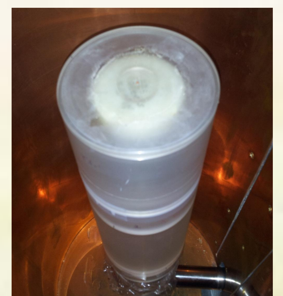
BEGe(Broad Energy Germanium, relative efficiency : 38%) detector system with the test sample
