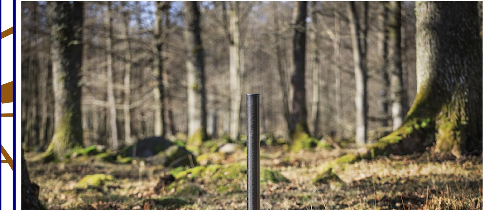
To simplify transport of the system and to protect it from the elements, it is placed within a water tight carbon fiber tube.
