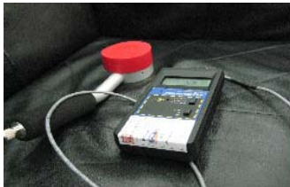
Fig 1. Surface contamination monitor (Type of detector : G-M tube, Model : Inspector/R, Company : S.E. International)
