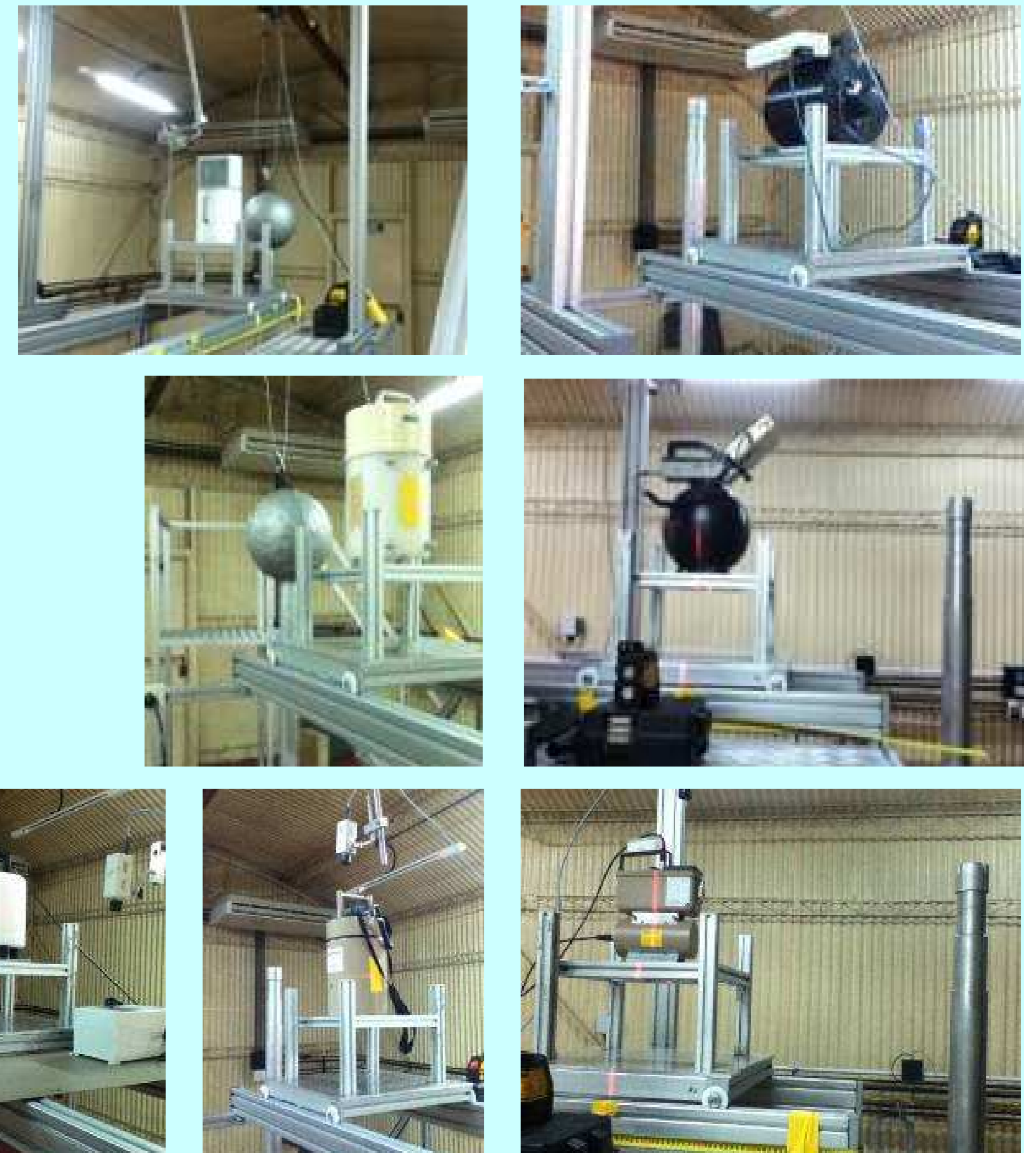
Figure 2. Detectors on calibration bank in the same positions as they were irradiated.
