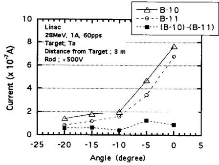
Fig. 2 Angular dependence of output currents of both  $^{10}\text{BF}_3$  and  $^{11}\text{BF}_3$  chambers operated around a target of an electron linear accelerator. The subtracted data correspond to the neutron component.
