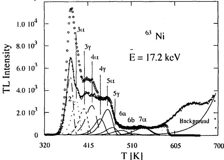
Figure 3. Glow curve of TLD-100 following <sup>63</sup>Ni beta irradiation
