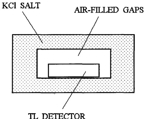
Figure 1. Schematic diagram for detector calibration exposure
