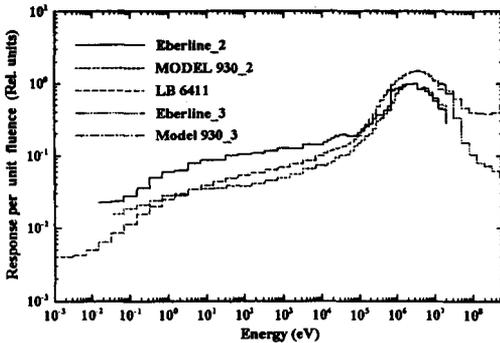
Figure 3. Survey instrument responses as a function of incident neutron energy. Eberline and Model 930 cf. ref. 7 and LB 6411 cf. ref. 8.
