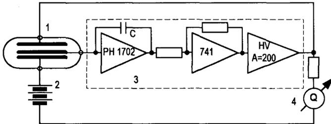
Figure 4. Functional circuit of the QF-meter: 1 - recombination chamber; 2 - high voltage source; 3 - high voltage electrometrical amplifier; 4 - voltmeter calibrated in units of quality factor.
