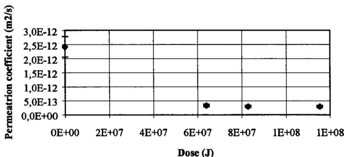
Figure1. Evolution of the permeation of radon in PVC versus UV dose
