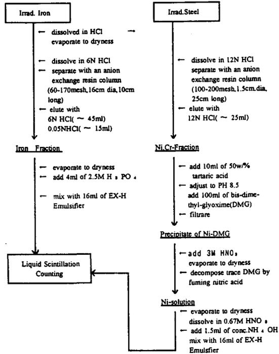
Fig.1 Procedures for chemical separation of  $^{56}\text{Fe}$  and  $^{63}\text{Ni}$  from irradiated iron and steel samples and preparation of counting samples for LSC
