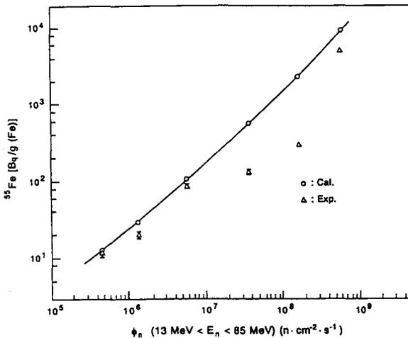
Fig.2 Relation between  $^{55}\text{Fe}$  activity [ Bq/g(Fe) ] and neutron fluxes
