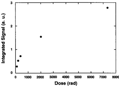
Figure 3: Dose response of the laser-heated, fiber-optic-coupled dosimeter.
