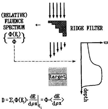
FIG.4 GEOMETRY OF SIMULATION
