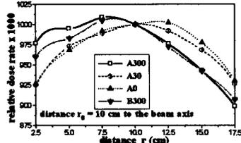
figure 4. PLD in front water phantom for different filtrations at 300 kV
