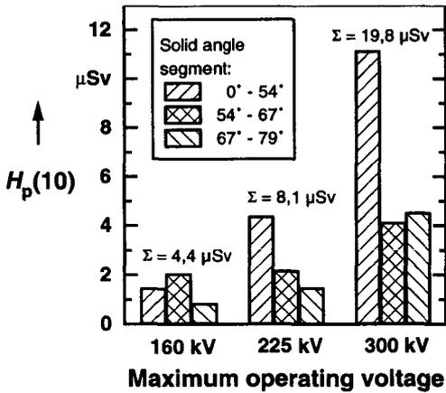
Figure 2. Angular distributions of the personal dose equivalent  $H_p(10)$  during the type testing of three different X-ray emitters (X-ray tubes with maximum operating voltages of 160 kV, 225 kV and 300 kV).  $\Sigma$  denotes the total dose measured during the respective type tests.
