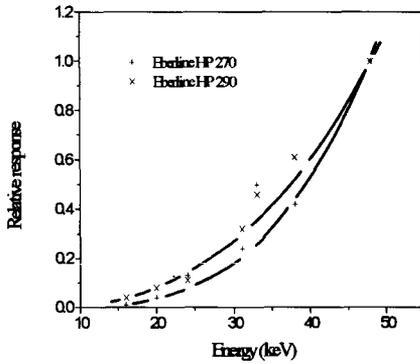
Figura 3 - Energy dependence of Geiger-Müller detectors
