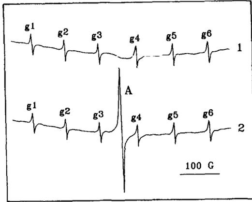
Figure 1. ESR spectra from virgin MgO:Mn, Fe single crystals (1) and crystals subjected to special thermochemical treatment (1) after (2) and before (2) UV or X-ray irradiation.
