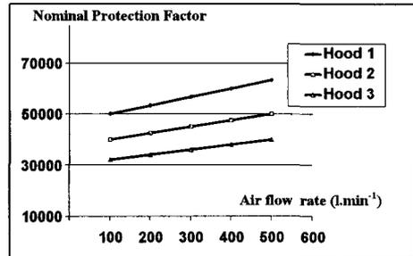
Figure 2 : Variation of NPFs by increasing air flow rate in ventilated-pressurized hoods.
