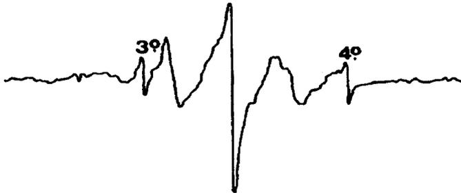
Figure 1. ESR spectrum of alanine irradiated with  $^{60}Co$  gamma rays at 1 kGy<sup>3</sup>.
