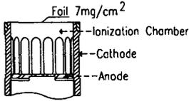
Fig. 1a DL 1 with original ionization chamber
