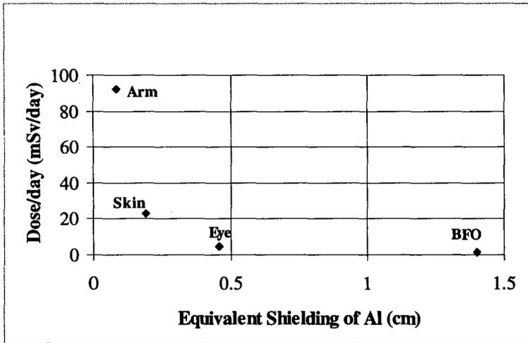
**Figure 2** Simulated dose level for an Astronaut in EVA for the proposed Alpha Space Station orbit.
