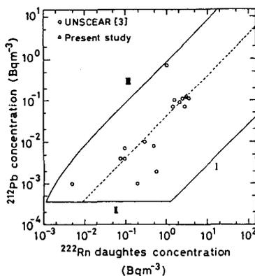
Figure 2. Zone where simultaneous measurement of  $^{222}\text{Rn}$  daughters and  $^{212}\text{Pb}$  is possible.
