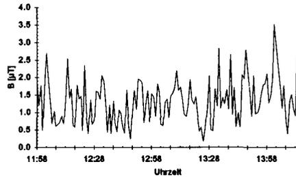
Fig. 5: Typical long-time measurement of magnetic field strength along a railway line in Berlin-Buch/Karow measured 1 m over ground at a distance of 12 m.
