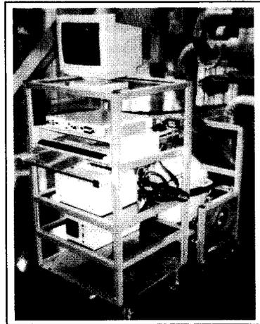
Fig. 6 The Noble Gas Compliance Monitoring Cart
