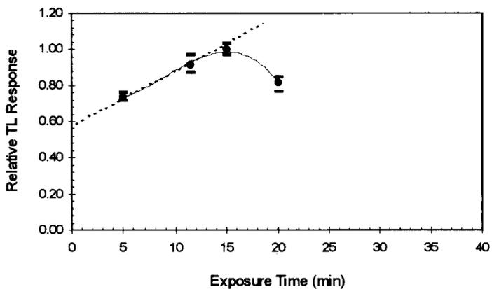
Figure 2. Dependence of TL Response as a Function of the Laser Exposure Time for CaSO<sub>4</sub>:Dy
