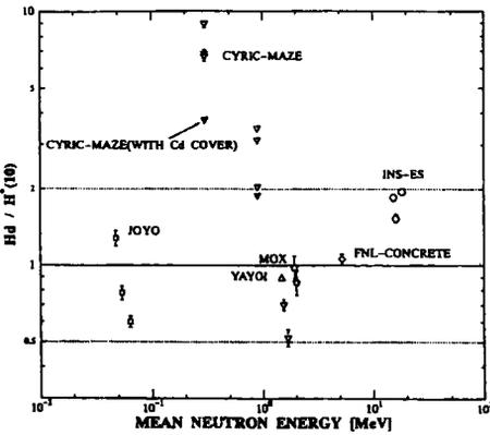
Fig. 9 Comparison of dose equivalent given by the Si dosimeter to that by the rem counter for various neutron fields having different mean neutron energies
