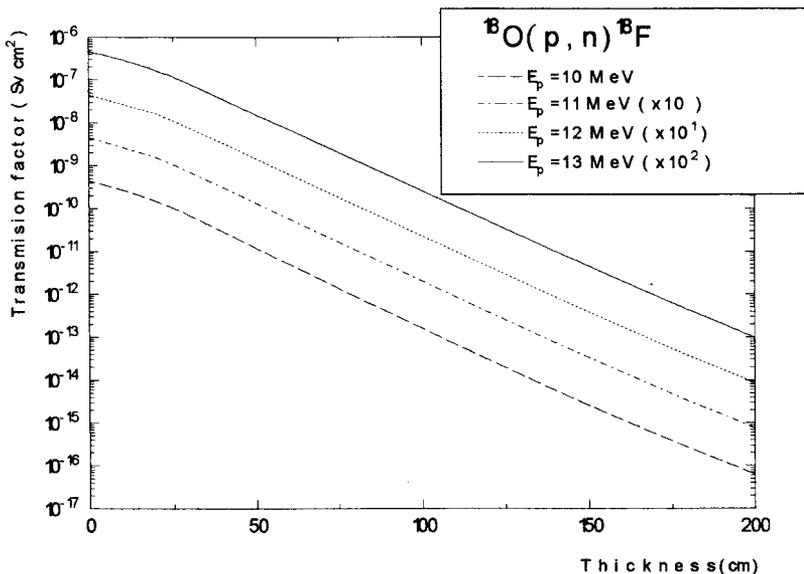
Figure 1: Transmission factors for the reaction  $^{18}\text{O}(p,n)^{18}\text{F}$ .
