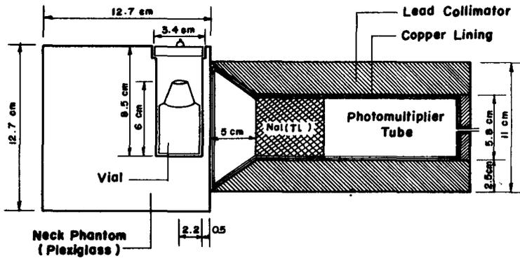
Fig. 1 The schematic diagram of the detector inside the collimator designed and constructed at the NRPD, AEOI.
