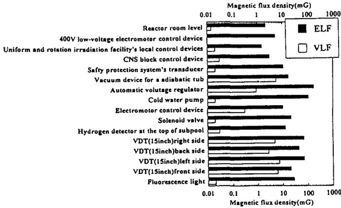
Figure 1. Magnetic flux density produced by electrical devices.
