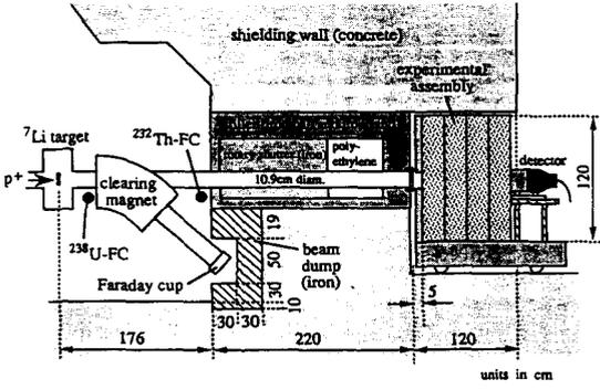
Fig. 4 Cross sectional view of the shielding experiment at TIARA
