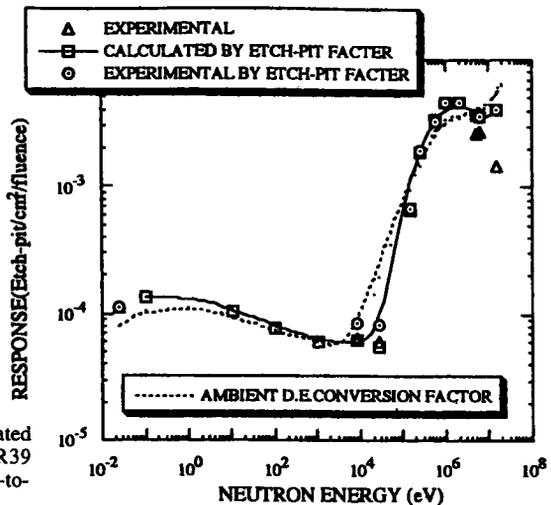
Fig.10 Comparison of measured and calculated neutron detection efficiencies of the CR39 dosimeter, together with the ICRP-51 fluence-to-dose-equivalent conversion factor
