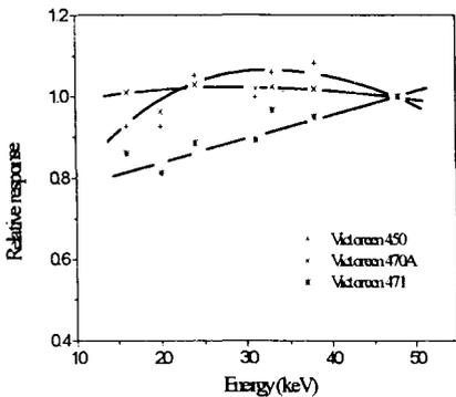
Figure 2 - Energy dependence of ionization chambers
