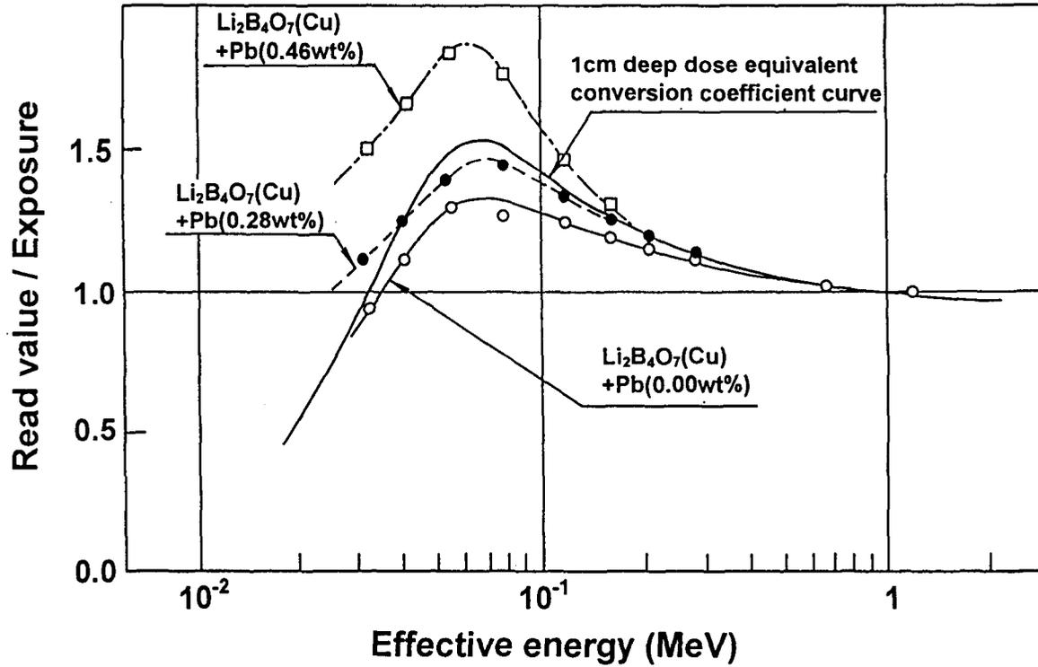
Fig.3 Energy response of  $\text{Li}_2\text{B}_4\text{O}_7(\text{Cu}, \text{Pb})$  TLD located on phantom
