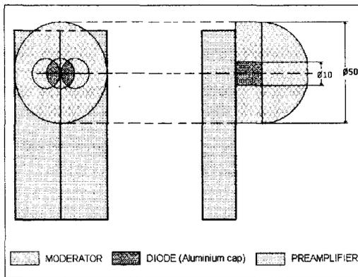
Fig.1. The detection assembly with moderator.
