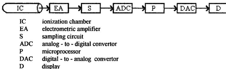
Fig. 2 - Block scheme of the functional model
