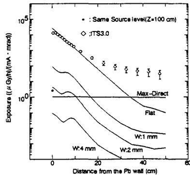
Fig.2 Dose distribution due to ground shine on the floor outside the hutch. (Photon source is scattered photons in  $90^\circ$  direction by Cu at 2m from scattered point. W denotes width)
