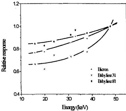
Figure 1 - Energy dependence of ionization chambers
