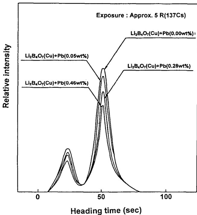
Fig.1 Glow curves of  $\text{Li}_2\text{B}_4\text{O}_7(\text{Cu})$  added with Pb
