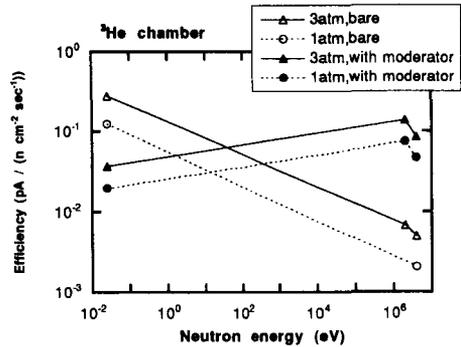
Figure 3. Response characteristic of  $^3\text{He}$  chamber against neutron energy.
