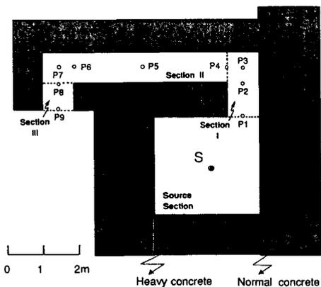
Fig. 1. Structure of labyrinth in cobalt-60 irradiation facility.
