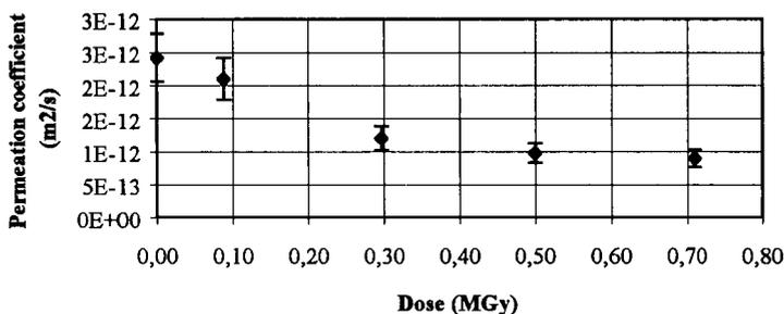
Figure 2. Evolution of the permeation of radon in PVC versus gamma dose (dose rate : 1,05 k Gy.h<sup>-1</sup>)
