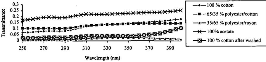
Fig. 4 Spectral transmittances of different types of fabrics
