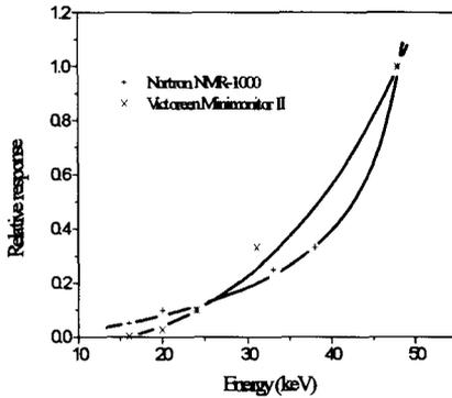
Figura 4 - Energy dependence of Geiger-Müller detectors
