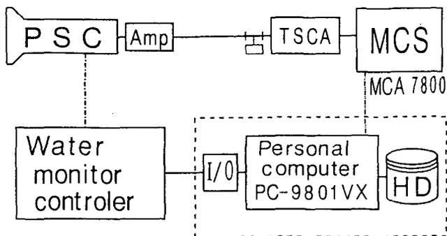
Fig.1. A schematic diagram of the computerized water monitor equipped with a plastic scintillator.
