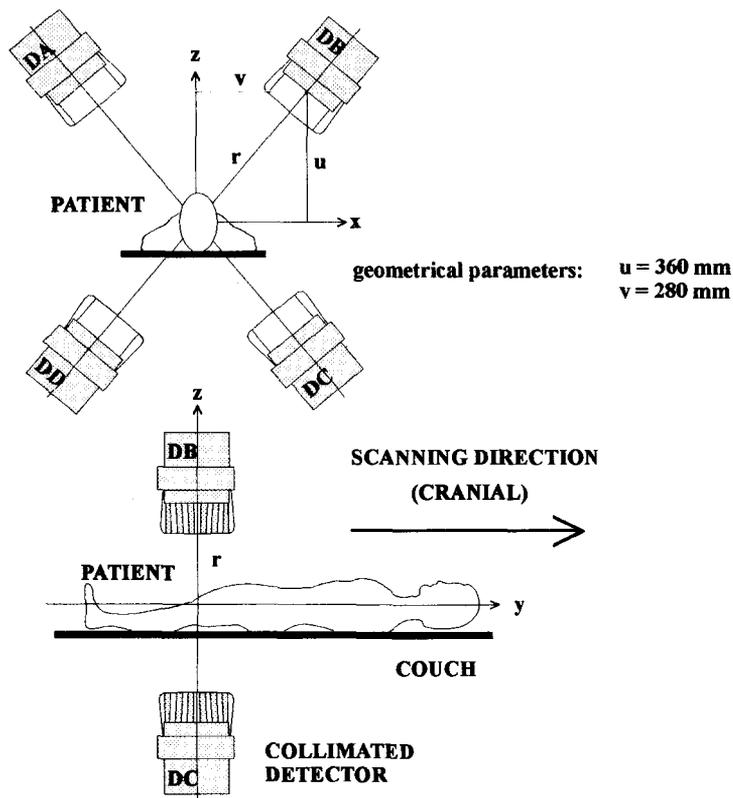
Fig. 1. Detector configuration.
