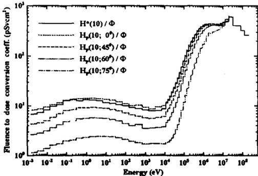
Figure 1. Neutron fluence to dose equivalent conversion coefficients<sup>(5)</sup> as a function of incident neutron energy.
