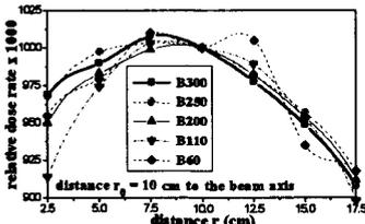
figure 5. PLD in front PMMA phantom for different tube voltages
