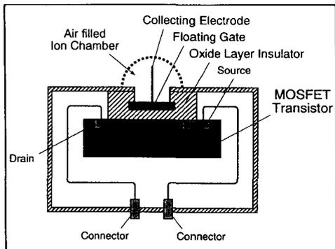
Figure 1. Schematic of a dosemeter based on DIS
