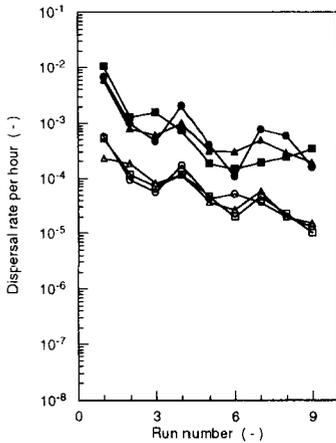
Fig.3 Effects of low and high dust loading on reentrainment of Pu particles at inverse flow of  $1.2 \times 10^2$  mm/s ( $\circ$ : continuous flow,  $\triangle$ : intermittent flow,  $\square$ : mechanical shock flow, open symbol: low loading, solid symbol: high loading)
