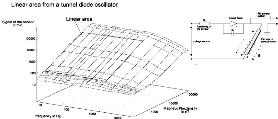
Fig. 4: Linear range from a tunnel diode oscillator
