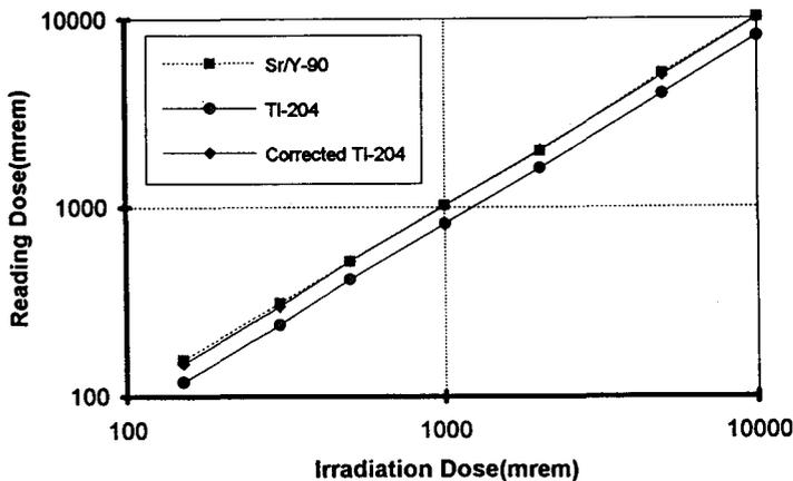
Figure 1. Linearity of Sr/Y-90 and Tl-204 Beta Particles.
