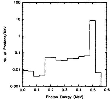
**Fig. 5** Transmitted photon spectrum of Na-22 through aluminium foil whose thickness is equal to the range of the endpoint energy of Na-22.
