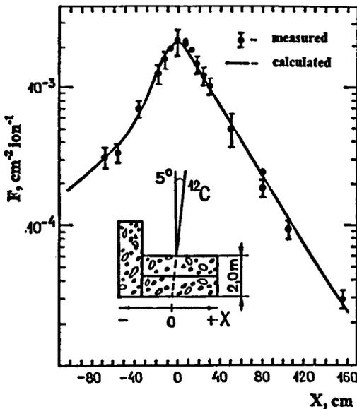
Fig. 3. Measured[27] and calculated[26] lateral distribution of high energy hadron fluence outside the beam stopper of  $^{12}\text{C}$  3.65 GeV/nucleon.
