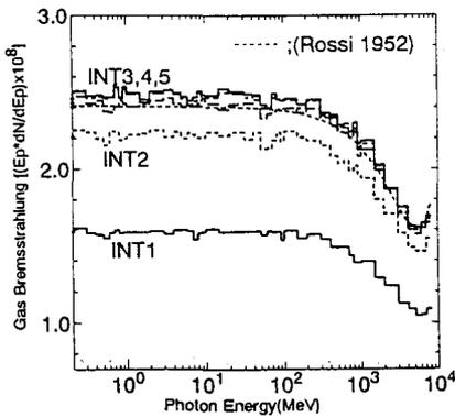
Fig.3 Gas bremsstrahlung spectra depending on the number of the interactions generated by EGS4 resulting from 0.1A 8GeV electron and interacting with 0.1205g/cm<sup>2</sup> air. (INT1;single interactions, INT2;double interactions, INT3.4.5; triple or more interactions, ---;theoretical data<sup>(8)(9)</sup>)
