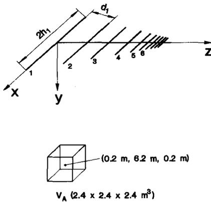
Fig. 1: Geometry of the logarithmic-periodic antenna
