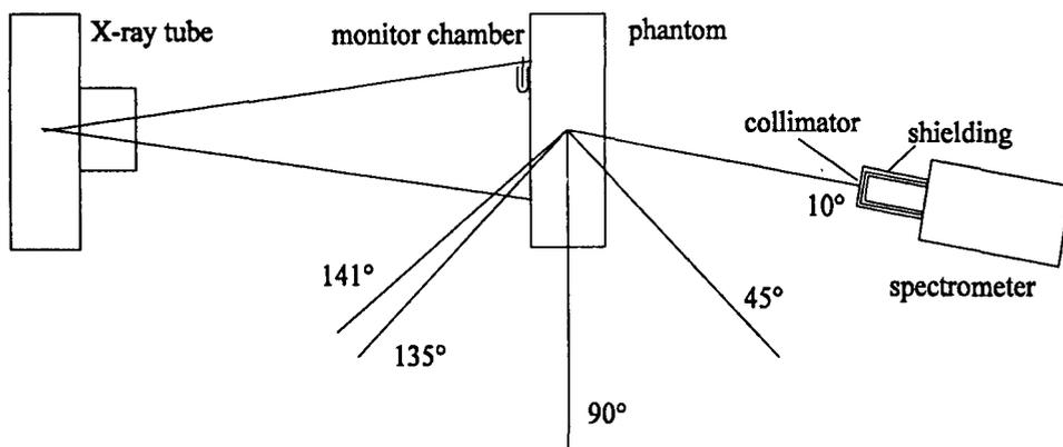
Figure 1. Experimental arrangement
