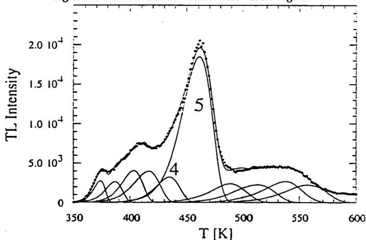
Figure 2. Glow curve of TLD-600 following fast-neutron irradiation
