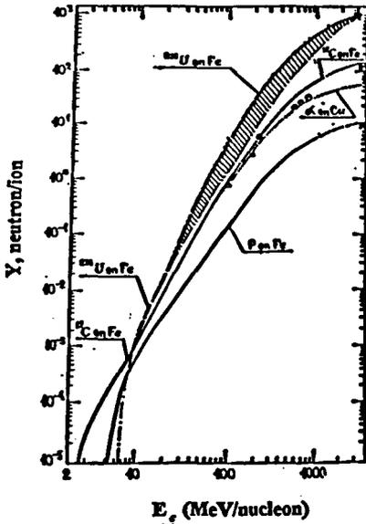
Fig. 1. Total neutron yield from the thick iron or copper target per one ion with energy of  $E_0$ .
