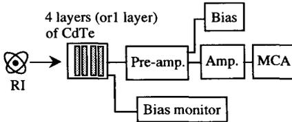
Fig. 5. Block diagram of the experiment.
