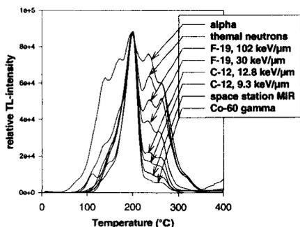
Fig.1: Glowcurves from TLD-600 after absorption of radiation with different LET (low dose)
