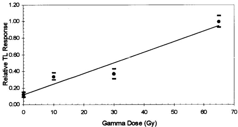
Figure 1. Dependence of TL Response as a Function of the Gamma Dose for CaSO<sub>4</sub>:Dy
