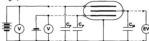
Figure 3. Self-contained measuring system. Broken lines show connections performed before and after irradiation.
