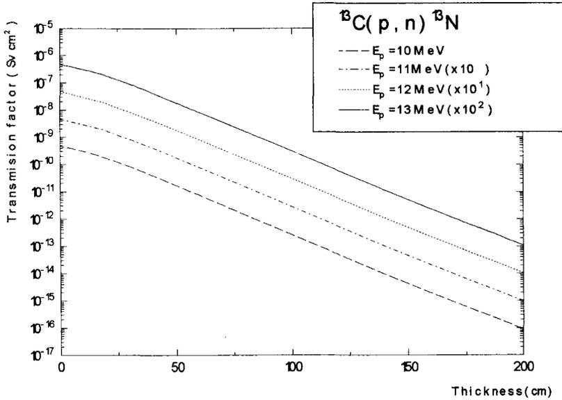
Figure 2: Transmission factors for the reaction  $^{13}\text{C}(p,n)^{13}\text{N}$ .
