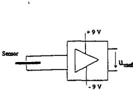
capacitive sensor 72 mm diameter, 125 pF
