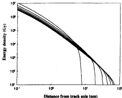
Fig 4: Calculated radial energy density in an alpha track. The distribution of energy density was calculated in 7 layers from the surface to the end of the range.
