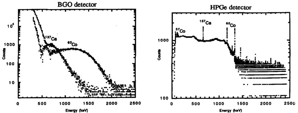
Fig. 3 Left: Separate Gamma Spectra obtained with BGO detector for  $^{60}\text{Co}$  and  $^{137}\text{Cs}$  sources
