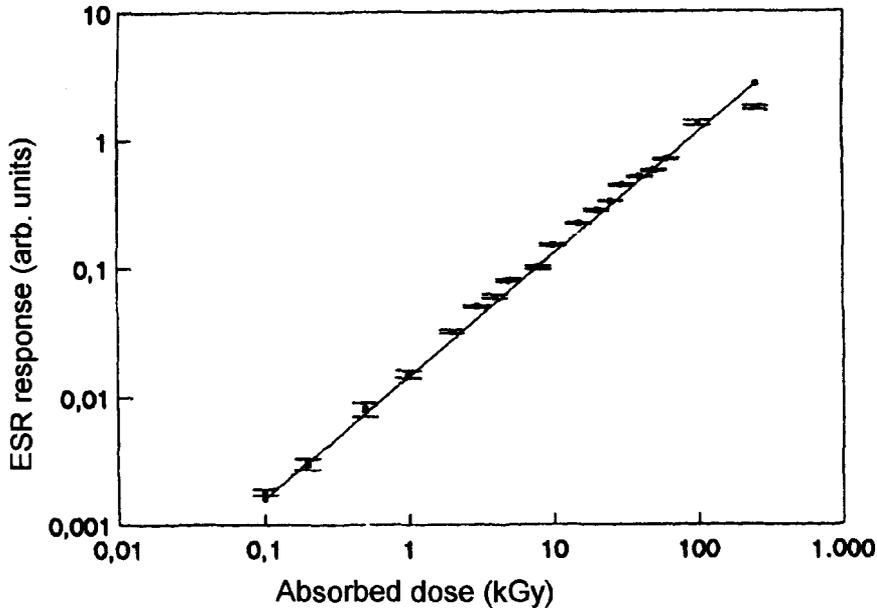
Figure 2 .Dose-response curve of DL-alanine irradiated by  $^{60}\text{Co}$  gamma rays<sup>3</sup>.
