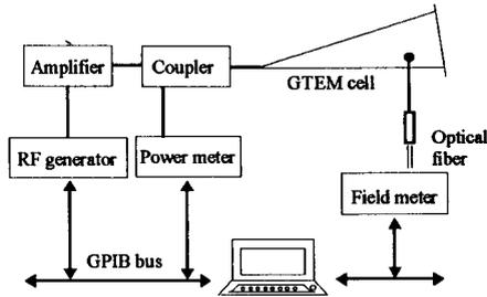
Fig. 3: Electric Field measurements test set up.
