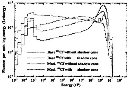
Figure 2. Calibration spectra in a bunker room<sup>(6)</sup> as a function of incident neutron energy.
