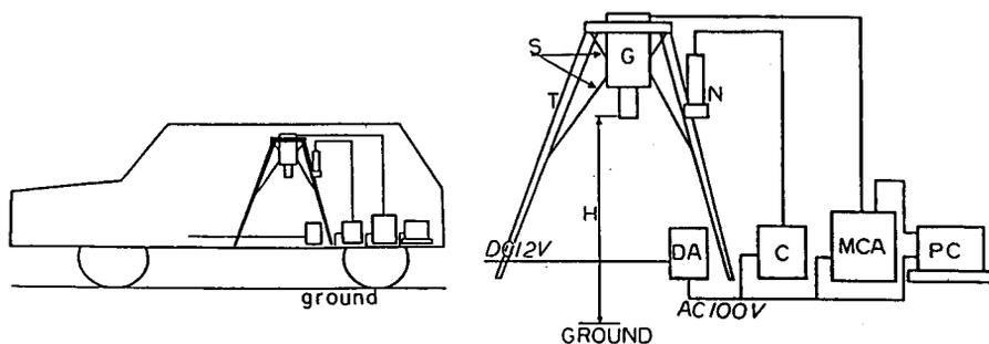
T: Tripod G: HPGe detector N: NaI detector DA: DC/AC inverter C: Controller MCA: Multi-channel analyzer
