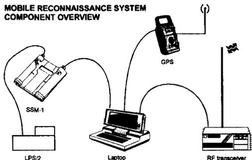
and timing coordinates. A RF-transceiver digitally broadcasts position and measurements as well as messages to the headquarter and relays commands to the field team. The headquarter may track up to 3 field teams simultaneously and communicate up to a distance of approximately 40 km. All data are stored internally in case of communication failure.
