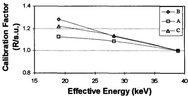
Figure 3. Energy Dependence of the IPEN parallel plate ionization chambers. All values were normalized to 50 kV to make easy the comparison.
