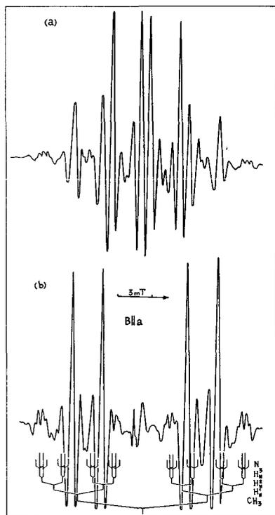
Fig. The spectra ESR  $\gamma$ -irradiated L-alanine single crystals: at  $T=293\text{K}$  (a); at  $T=160\text{K}$  (b)
