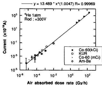
Figure 2. Responses to gamma rays, (1 atm  $^4\text{He}$  chamber).
