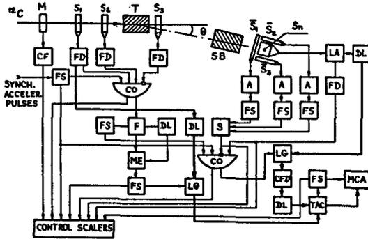
Fig.5 The experimental arrangement and block diagram of the TOF spectrometer. LC - linear gate, CFD - constant fraction discriminator, TAC - time-to-amplitude converter, FS - fast logic shaper, S - logic summator, ME - multiple events unit, F - fanout unit, M - beam monitor chamber, T - target, CF - current-to-frequency converter, SB - shadow bar, A - fast amplifier, LA - linear amplifier, DL - delay unit, FD - fast discriminator, CO - coincidence unit, MSA - multichannel analyzer.
