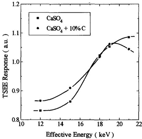
Figure 3. Energy dependence of CaSO<sub>4</sub> sintered pellets.
