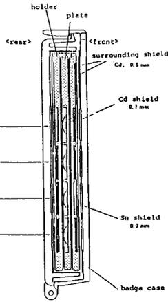
Fig.1 Cross-sectional view of PNC/Panasonic albedo TLD (type; UD-809P)
