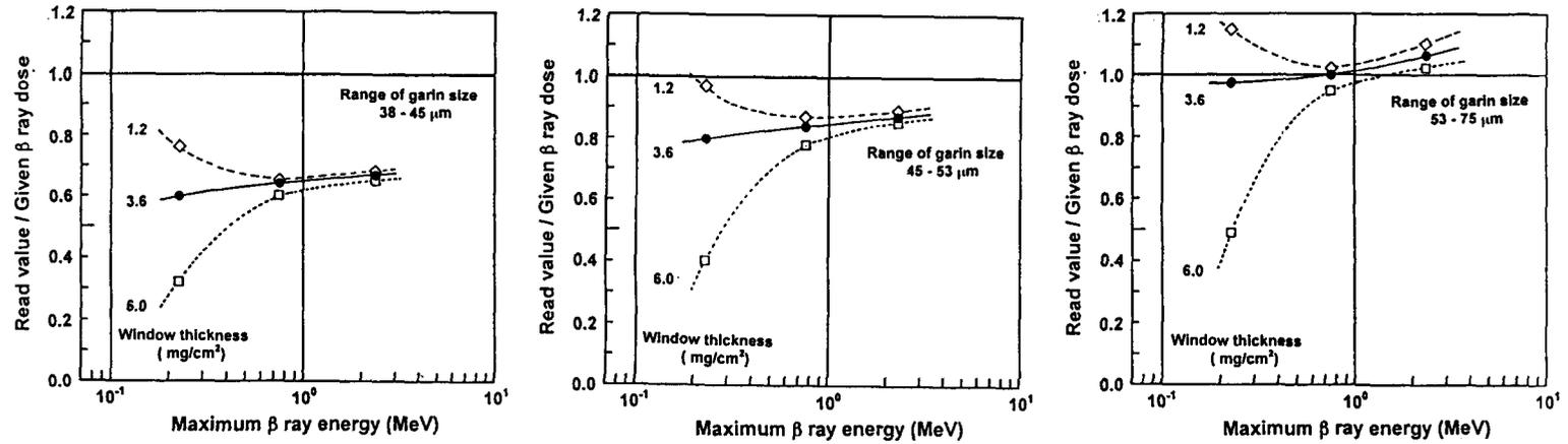
Fig.1 Response of the single layer of the  $\text{Li}_2\text{B}_4\text{O}_7(\text{Cu})$  grains covered with polyethylene film of various thickness.
