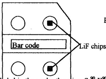
Fig. 1: Schematic of a TLD card used by the Harshaw 6600 System.
