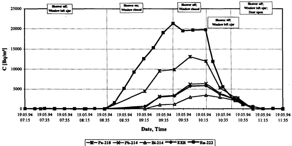
Figure 1 Rn-222- and Rn-222 Daughter Nuclides Concentration in Air while Taking Showers (Volume 11,25 m<sup>3</sup>; Rn 222 concentration in Water 685 Bq/l; 9 °C; 15 - 18 l/min)
