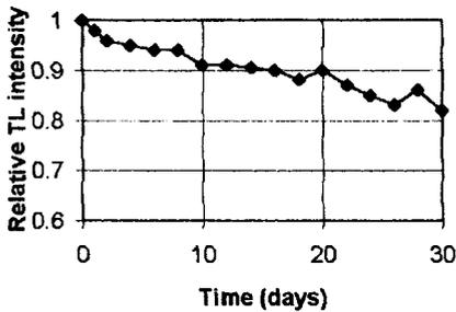
Fig. 2: Fading of TL chips used by Harshaw 6600
