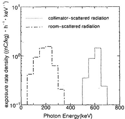
Figure 2 The spectral distribution of exposure of scattered radiation in the small room with <sup>137</sup>Cs source. The source-to-detector distance is 2.0m.
