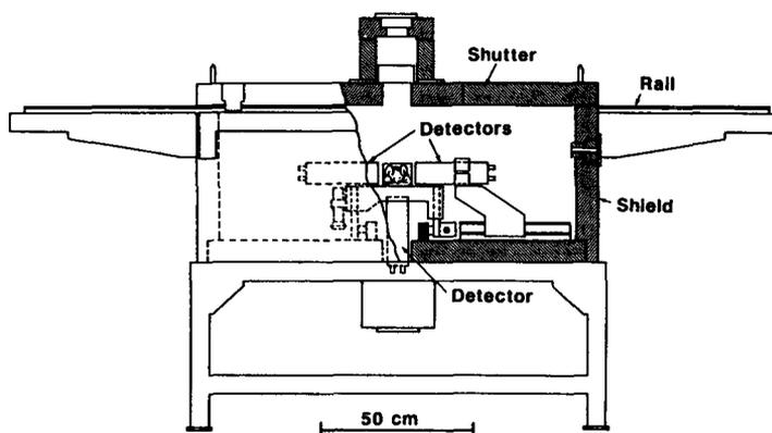
Figure 1. Schematic diagram of the whole-body counter.
