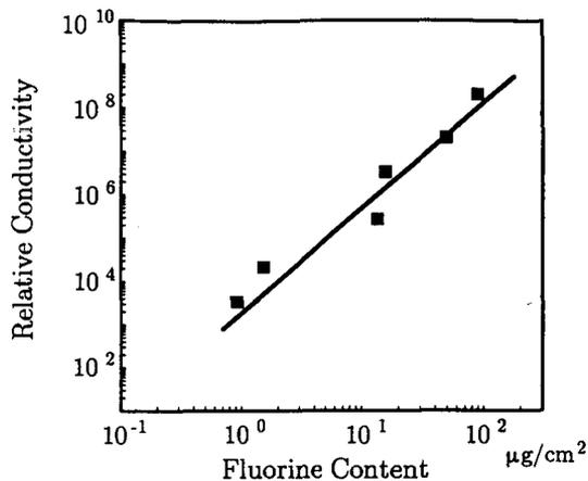
Fig.2 Relationship between the fluorine content of the polyaniline film and the conductivity
