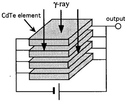
Fig. 1. Multi-layered CdTe detector.
