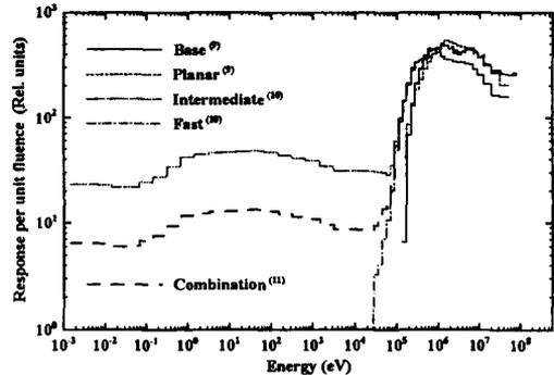
Figure 4. Etched track dosimeter responses<sup>(9,10,11)</sup> as a function of incident neutron energy.
