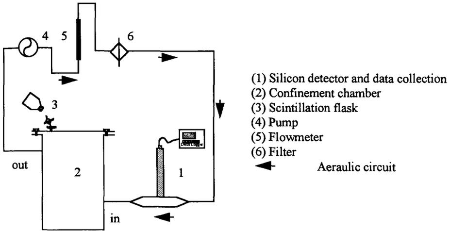
Figure 1 - Testing Apparatus
