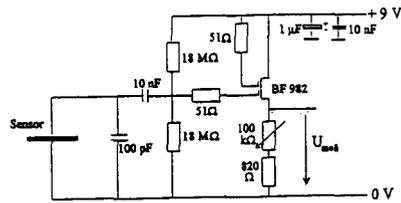
capacitive sensor 72 mm diameter, 125 pF
