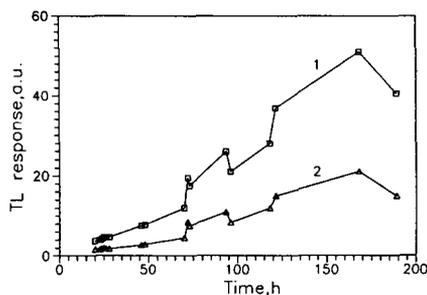
Figure. TL response vs. self-irradiation time of two BeO:TiO<sub>2</sub> ceramic detectors
