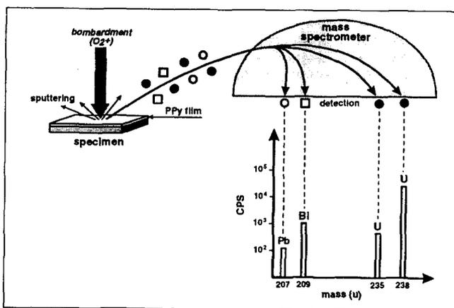
Figure 1 - Schematic representation of SIMS physical principles.
