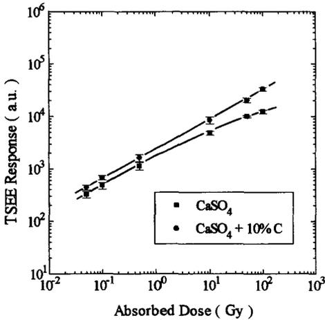
Figure 2 . The TSEE response for  $\text{CaSO}_4$  sintered pellets.
