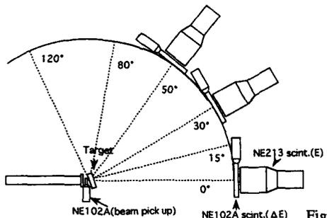
Fig. 6 Schematic diagram of the thick-target yield experiment at HIMAC
