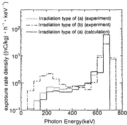
Figure 1 The spectral distribution of exposure for the two irradiation types of (a) and (b) in the small room with <sup>137</sup>Cs source. The source-to-detector distance is 2.0m.
