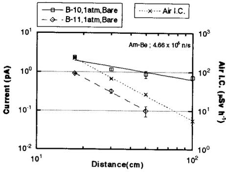
Fig. 1 Dependence of output currents of both  $^{10}\text{BF}_3$  and  $^{11}\text{BF}_3$  chambers on distance in the  $n-\gamma$  mixed field of Am-Be neutron source. The dose equivalent rate due to  $\gamma$ -rays measured with ionization chamber is also shown.
