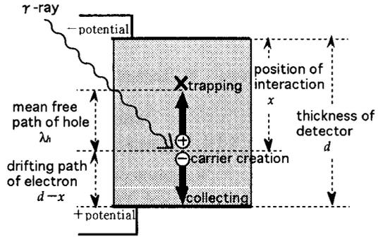
Fig. 2. Simulation model considering the hole trapping in the semiconductor detector.
