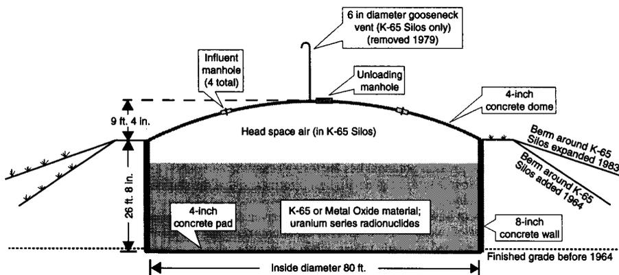
Figure 1. Schematic diagram of the K-65 silos located on the Fernald site.
