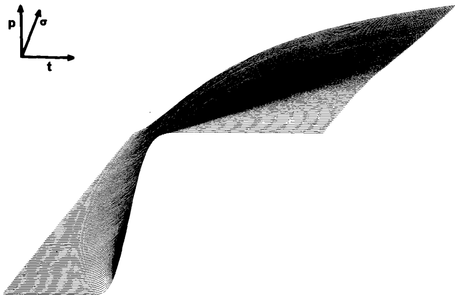
FIGURE 8: Integrated log-normal probability density distribution with constant median at 0.4 of the time scale and \sigma increasing linearly from 0.1 (front) to 1.0 (back).
