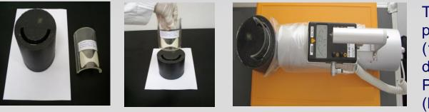
The neck phantom: polyethylene cylinder (11.4 cm diameter and 11.3 cm high), developed by Institute of Radiation Protection and Dosimetry of Brazil (IRD) in the frame of Project IAEA/ARCAL RLA 9/049.
