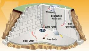
Seal major entry routes for radon such as sump holes, cracks in foundation and exposed soil and rock in crawlspaces.
