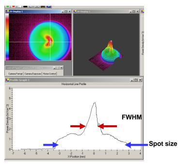
Because of the "hot spot", the 50% of the peak (FWHM) criterion is much smaller than the spot size
