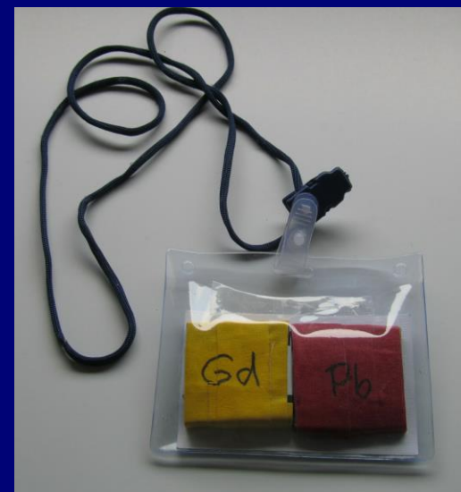
The WPE Albedo Dosimeter Badge (rear view)
