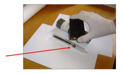
The oldest man-made source used in Slovenia was <sup>226</sup>Ra source of 0.15 MBq produced in 1902 and used in ophthalmology. Later it was lost for decades. In 2007 it was found in an abandoned storage during the SNSA inspection programme of finding non-registered sources in the state.
