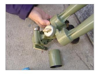
A typical old military item with non-registered <sup>226</sup>Ra source inside it. No label related to radioactivity was used at the time the equipment was acquired.
