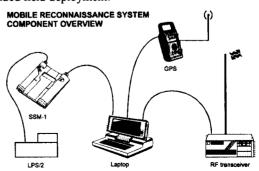
and timing coordinates. A RF-transceiver digitally broadcasts position and measurements as well as messages to the headquarter and relays commands to the field team. The headquarter may track up to 3 field teams simultaneously and communicate up to a distance of approximately 40 km. All data are stored internally in case of communication failure.
